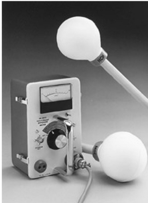
Fig. 8. Electric and Magnetic Field meter. Readout device is same for E and M probes
